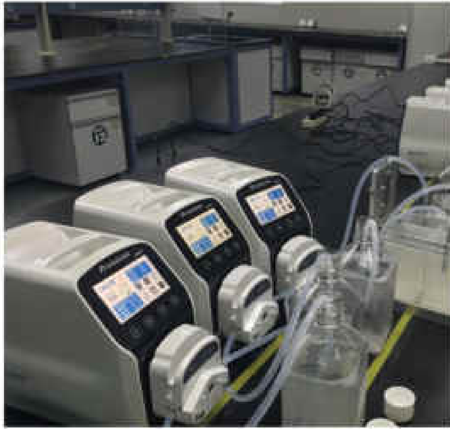
Laboratory chemical dosing
