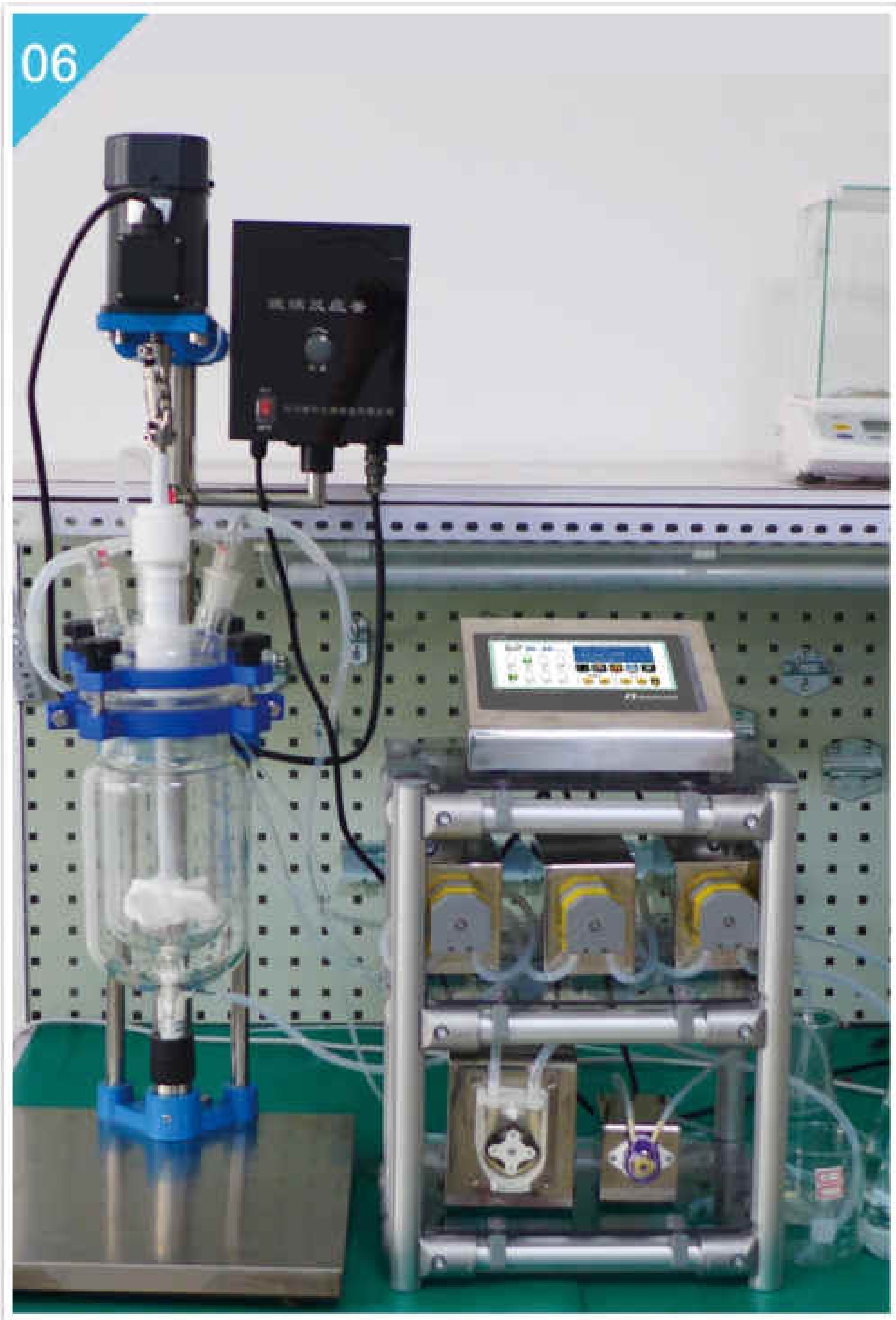
06 Bio-pharmaceutical Work with reactor or fermentation tank, the OCM system add different liquids with proportion and order into reactor. Together accomplish adding liquid, mixing, reaction, dispensing, waste discharge and washing function.
