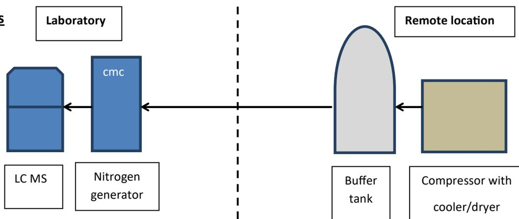
Where no in-house compressed air supply is available cmc Instruments recommend a remote compressor and buffer tank. The heavy duty compressor has a low load and needs to run for less than 25% of the time in normal duty. An integral cooler/dryer ensures there is no moisture in the resultant compressed air. This mode of operation results in low maintenance on the compressor, typical interval to first service is 2.5 years. Buffer tanks are available in three sizes dependent on air demand.
